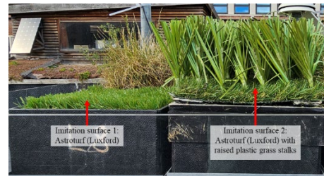
Figure 2 – Imitation surfaces: left – Wickham et al. (2025); right – modified surface. The modular cells sit on aluminium trays connected to the load cells.
