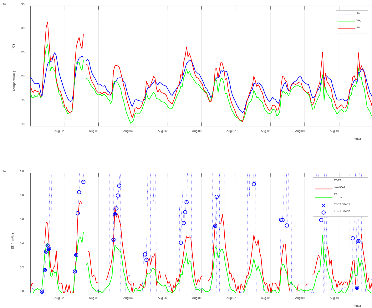
Figure 3 – Time-series of a) Temperature and b) ET_o , Measured ET (load cells) and ET estimated using the 3T method for 10 days in August 2024
